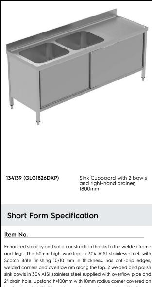
the back with AISI 304 stainless steel spot welded profile. Square section legs and height adjustable feet (-20 +30 mm) in 304 AISI stainless steel. 40 mm-thick lower welded shelf in AISI 304 stainless steel slots easily into place at a height of 200 mm from the floor (compulsory toinstall the chest of drawers).Square section legs and height adjustable feet (-20 +30 mm) in 304 AISI stainless steel.
